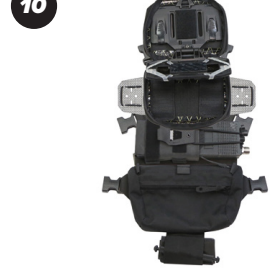
PTT Wings and MOLLE velcro tab are inserted into back of FlipLite Jacket. Radio Cables are routed to FlipLite device
